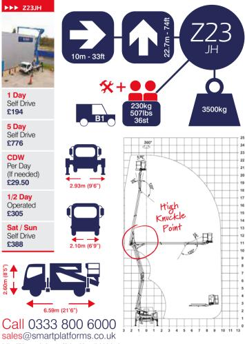
Jacking width is measured to the centre of the leg and does not include jack pads. All specs serve as a guideline only and are correct at the time of going to print. Smart reserve the right to change the specification without any prior notice.
